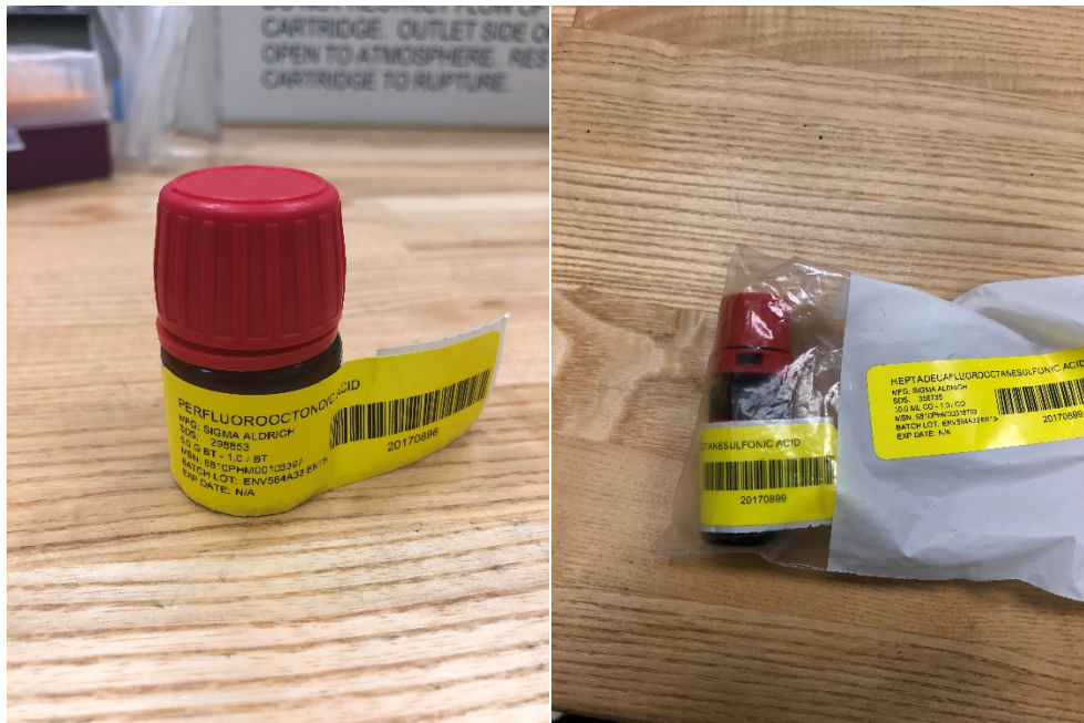
Figure 3-1: Original forms of PFAS solutions. PFOS (left) began as a 40% solution in water while the PFOA (right) was a 96% pure crystal form.
